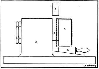
Fig. 36. Fixture for Trimming Edges of Drawn Parts
